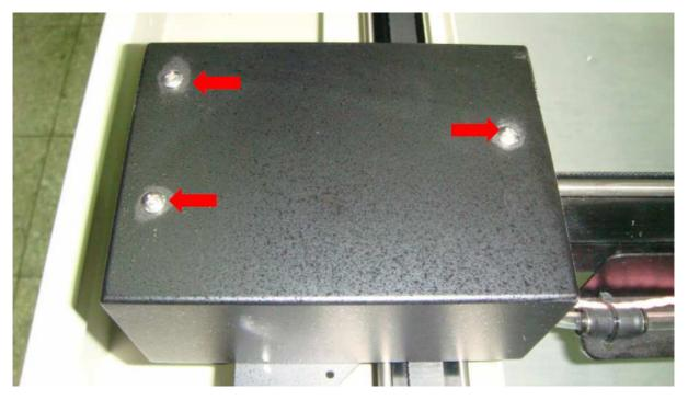
4-1. Dismount 3 screws of x motor idle pulley (Blue circle below). Dismount 4 screws of X motor (M3 \*10,red arrow below) and the x motor cable be removed and changed.
