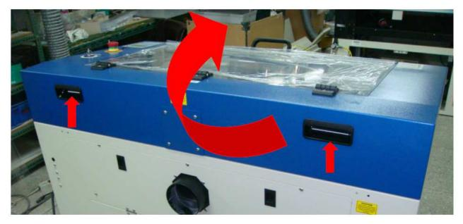
3. Please turn the safety lock switch to LOCK status according to the direction shown on the sticker (see picture) to avoid the collapsing of top cover.
