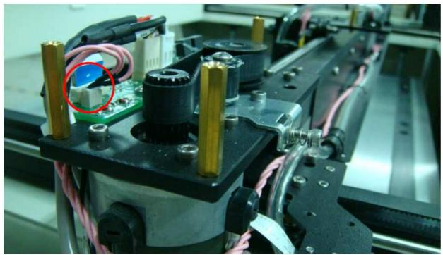
5-1. On lens carriage side, remove the auto focus cable also (it is tight, so use tweezers will be helpful).
