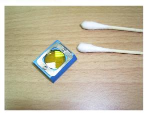
Make sure the lens is clean and dried before putting it back in the pen carriage unit.
