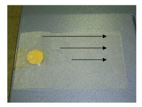
Make sure the lens is cleaned, dried and does not have any debris on the surface.
