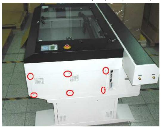
2. Dismount 7 screws (see red circles below) and remove all cables connecting to main board and can change new main board.
