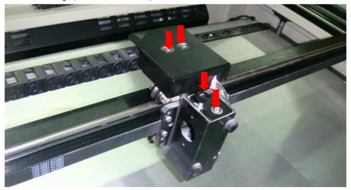
5. To change rollers, simply remove the hex bolts using a size 2 Allen key as shown below.
