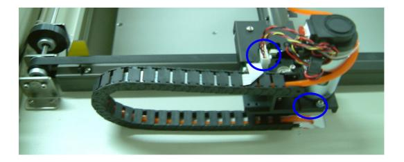
4. There are four screws on the bottom of x motor. Remove these four screws and the x motor can be removed and changed new one.
