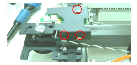
5. Remove three screws on x motor PCB cover.
