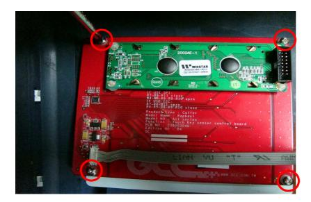
5. Withdraw Spacer Support from LCD Module.
