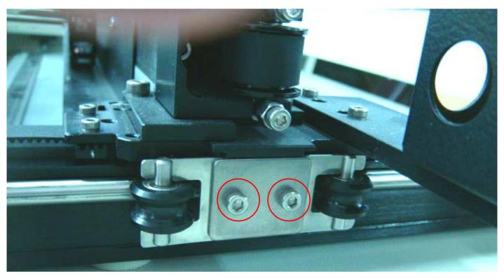
5. Unscrew the following screws to remove the A roller.
