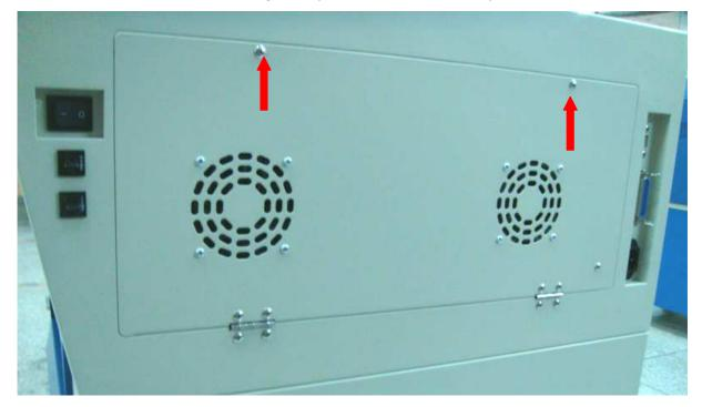
2. Dismount 4 screws (see red arrows below) and remove all cables connecting to main board and can change new main board.
