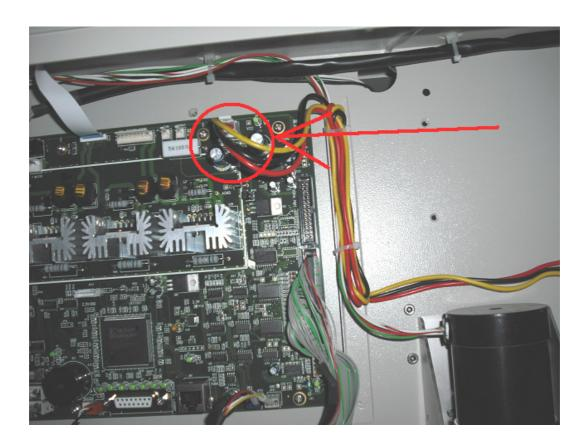
4. Loosen five screws to remove the power board (see picture below)
