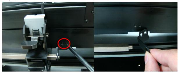
3. Push to right side; take out the Pinch roller from the slot on rail.
