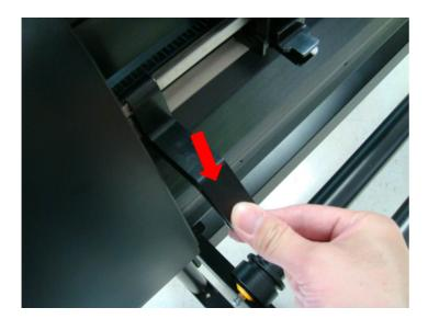
2. Behind of the machine, on right side use Phillips screwdriver to loose the screw shown as below picture and remove the metal racket.
