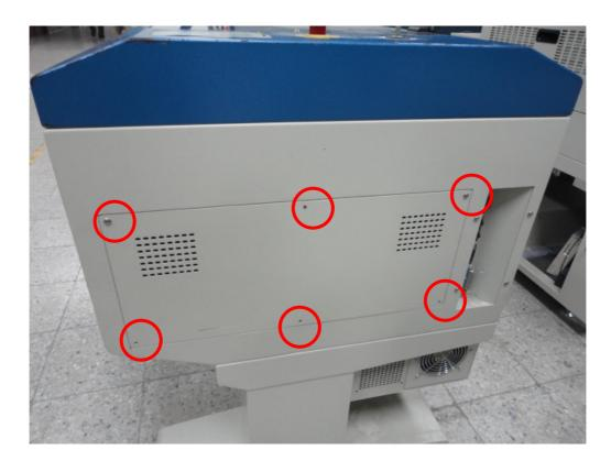
2. Dismount 7 screws (see red circles below) and remove all cables connecting to main board and can change new main board.
