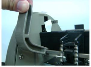
2. Behind of the machine, on right side use Phillips screwdriver to loose the screw shown as below picture.
