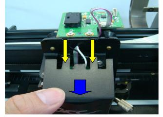
5. Use wrench to unscrew 2 nuts on the carriage.
