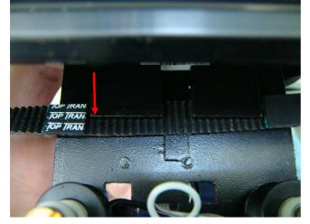
Belt completely set into groove.
