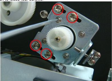
7. Change X motor and tension the belt back to the origin marked position.
