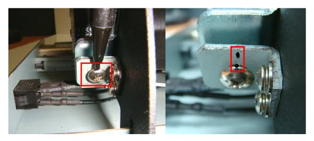
4. Use Phillips screwdriver to counter anticlockwise rotate screw **two** circles, release the belt. (Black mark is still aligned)
