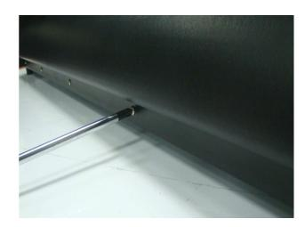
2. Use Slotted screwdriver to scrape off the glue on all connector.
