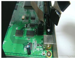
4. Use Phillips screwdriver to loose four screws on main board.
