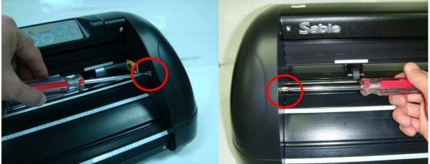
2. Use Phillips screwdriver to loose four screws on top cover.
