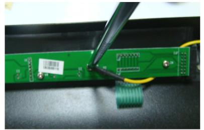
7. Use Slotted screwdriver to scrape glue and remove the screws.
