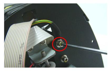
4. Use Slotted screwdriver to scrape off glue on flat cable connector.
