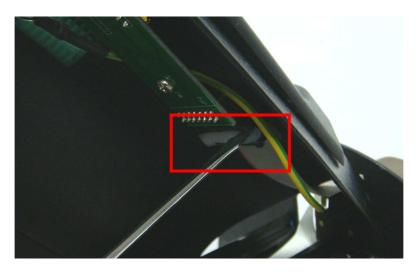
5. Pull out flat cable on control panel, and then remove the top cover.
