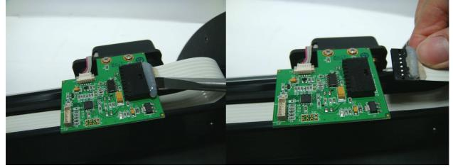
2. Use Slotted screwdriver to loose two screws on top of carriage from the back.
