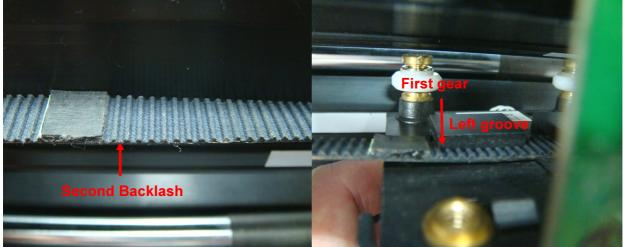
Belt completely set into groove.
