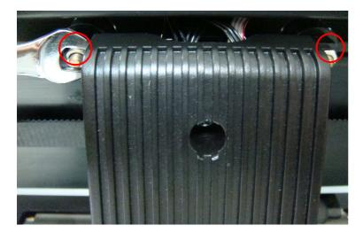
9. Use Slotted screwdriver to loose two screws on top of carriage from the back. (NOTE: loose it but not to remove).
